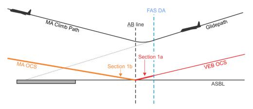
Figure 1 is an example where the RNP AR procedure design criteria limits construction where Section 1a sloping surface intersects the ground. The intent of the downward slope of Section 1a of the OCS beyond DA is to protect for a 50' height loss by the aircraft when the flight crew initiates a go-around at DA to begin the missed approach.
