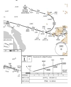
San Diego RNP RWY 27 has a MAS 1b controlling obstacle of a 309' (a pole) within the proposed level OCS segment. With application of the proposed new RNP AR criteria, the procedure designer can reduce the HAT for the RNP 0.11 line of minima from 617' to 453'.
