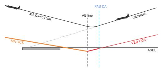
Figure 2 shows the existing surfaces with a HAT of 250'. The RNP AR vertical error budget's (VEB) OCS extends below the ASBL. Since the criteria prohibits a penetration of the OCS, the procedure designer using existing criteria must raise the DA so that the MAS OCS does not have a penetration.
