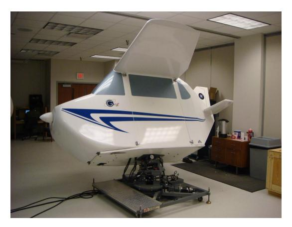
**GAT II HELO** is a basic Helo trainer that combines flight training, instrument training and spatial disorientation training in one low cost platform. The HELO GAT-II features an enclosed cockpit, realistic flight controls, and a wide-field-of-view. The 3 axes motion system is precisely coordinated with the visual display and the flight control inputs to provide a high fidelity learning environment. GAT-II HELO can be used at any time in any weather.
