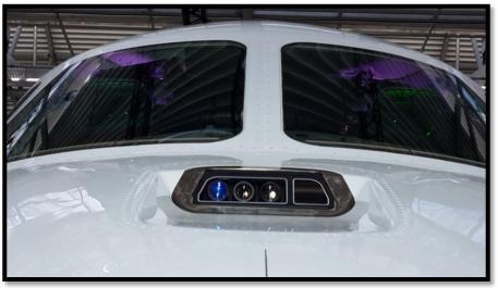
An EFVS includes the display element, sensors, computers, power supplies, indications, and controls.
