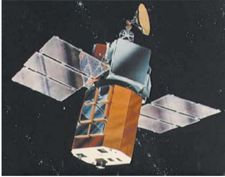
Figure 4.1.2-26. Solar Max Spacecraft. Spacecraft with large surface areas, such as solar panels, must correct for the pressure from solar radiation that may change their attitude. (Courtesy of NASA/Johnson Space Center)
