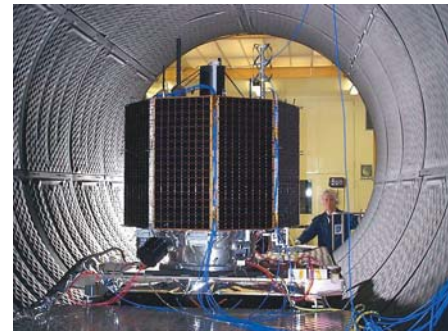
Figure 4.1.2-19. Spacecraft in a Vacuum Chamber. Prior to flight, spacecraft undergo rigorous tests, including exposure to a hard vacuum in vacuum chambers. In this way we can test for problems with out-gassing, cold welding, or heat transfer. (Courtesy of Surrey Satellite Technologies, Ltd., U.K.)
