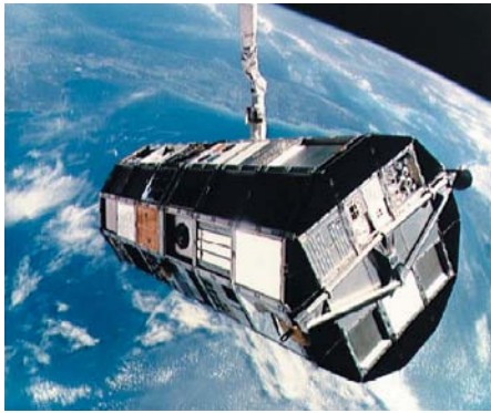
Figure 4.1.2-18. Long Duration Exposure Facility (LDEF). The mission of LDEF, deployed and retrieved by the Space Shuttle (STS-41-C) in April, 1984, was to determine the extent of space environment hazards such as atomic oxygen and micrometeoroids. (Courtesy of NASA/Johnson Space Center)
