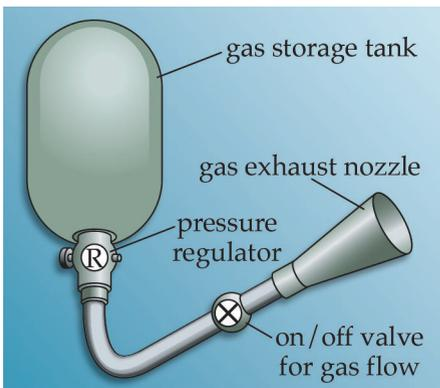
**Figure 4.2.1-12. A Cold-gas Thruster.** A cold-gas thruster is perhaps the simplest example of a rocket. In a typical thruster, shown in the cross-sectional drawing (upper), a gas enters from the right and stays behind the solenoid seal until it opens on command, releasing the gas through the nozzle. (Courtesy of Polyflex Aerospace, Ltd., U.K.)
