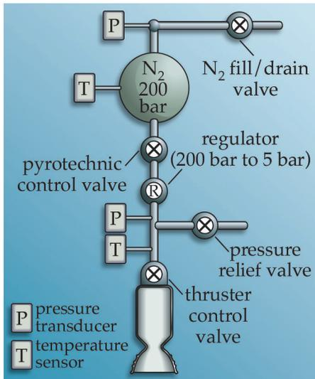
**Figure 4.2.1-20. FireSat's Propulsion Subsystem.** Even a relatively simple system such as a cold-gas thruster for a small satellite like FireSat requires tanks, valves, and sensors to measure and control the propellant flow.
