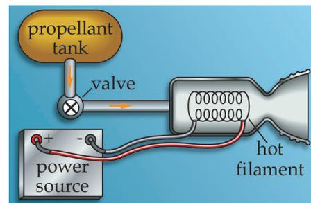
**Figure 4.2.1-31. Resistojet.** A resistojet uses electrical resistance to produce heat inside a thrust chamber. This heat transfers to the propellant by convection to the propellant flowing through the chamber, which then expands through a nozzle.
