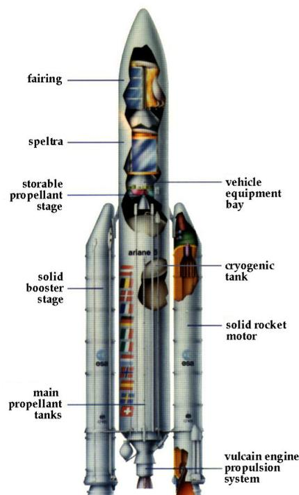
**Figure 4.2.1-55. Ariane V Cut-away.** Most of the mass and volume of this giant booster consists of propellant tanks. (Courtesy of Arianespace/European Space Agency/Centre National D'Etudes Spatiales)
