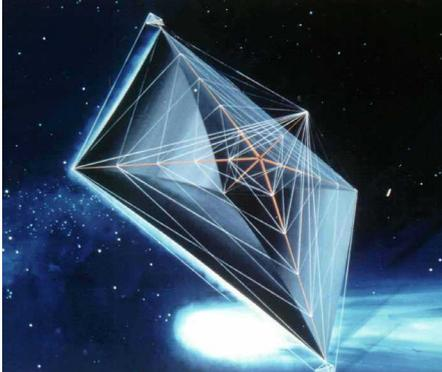
**Figure 4.2.1-44. Solar Sail.** A solar sail captures the minute pressure exerted by solar radiation. Even a very large surface area (1 km<sup>2</sup>) would generate only about 5 N of thrust. But this thrust is essentially “free” because no mass is expended. Thus, the solar sail is free to sail around the inner solar system (where solar radiation is most intense). (Courtesy of NASA/Jet Propulsion Laboratory)
