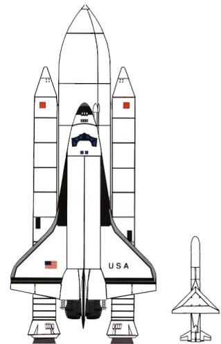
**Figure 4.2.1-50. Comparing Launch-vehicle Sizes.** Launch vehicles come in all shapes and sizes, from the massive Space Shuttle with a total lift-off mass of 2,040,000 kg to the tiny Pegasus (XL) at a mere 24,000 kg. (Courtesy of NASA/Johnson Space Center and Orbital Sciences Corporation)
