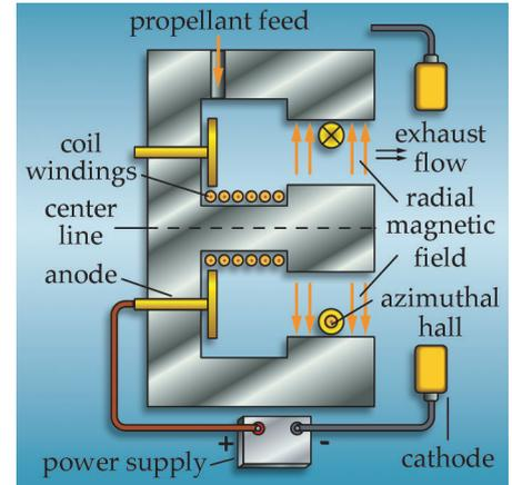
**Figure 4.2.1-39. Hall-effect Thruster (HET) Diagram.** In an HET, the interaction of an applied magnetic field with the resulting electric field creates the force that accelerates the positive ions within the plasma. This diagram shows a cross-section of the radial chamber.
