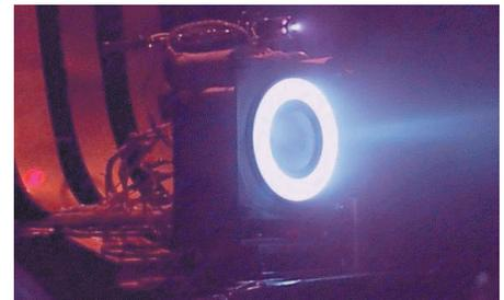
**Figure 4.2.1-40. Hall-effect Thruster (HET) in Operation.** Notice the circular shape of the plasma. HETs take advantage of the unique properties of a radial magnetic field to accelerate a propellant, such as Xenon, that has been heated to create a plasma. (Courtesy of Primex Aerospace Company)
