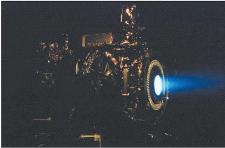
**Figure 4.2.1-43. Rocket Testing.** From initial development through flight testing, rockets and propulsion systems undergo rigorous testing to measure performance and ensure safe, reliable operations. This photograph shows the NSTAR ion thruster used for the NASA Deep Space 1 mission in its test-stand configuration. (Courtesy of NASA/Jet Propulsion Laboratory)
