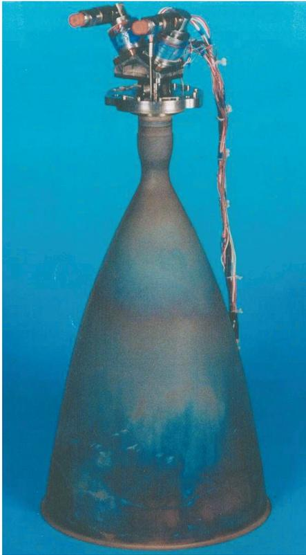
**Figure 4.2.1-23. LEROS Bipropellant Engine.** The LEROS engine, produced by the ARC Royal Ordnance in the United Kingdom, is just one example of a bipropellant rocket. It uses nitrogen tetroxide ( $N_2O_4$ ) with hydrazine ( $N_2H_4$ ) to deliver a total thrust of 400 N at 317 s specific impulse. This engine has been reliably used on a Mars mission and other deep-space and near-Earth missions for orbit insertion. (Courtesy of British Aerospace Royal Ordnance)
