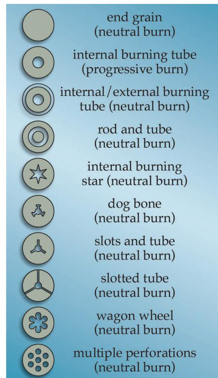
**Figure 4.2.1-25. Solid-propellant Grain Designs.** By altering the grain design, engineers cause progressive or neutral burn rates. Shaded areas indicate propellant, and blank areas indicate empty space. (Courtesy of Space Propulsion Analysis and Design by Humble, et al.)
