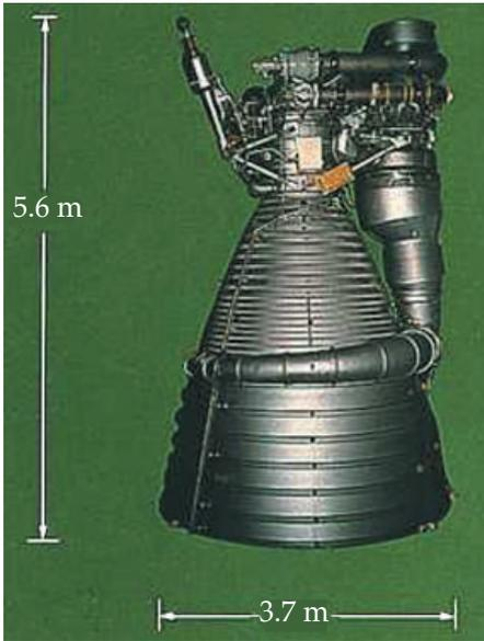
**Figure 4.2.1-8. Saturn V Nozzles.** Most rockets rely on nozzles to convert thermal energy into kinetic energy through thermodynamic expansion. We show the huge nozzles for the Saturn V F-1 engines here. (Courtesy of NASA/Marshall Space Flight Center)
