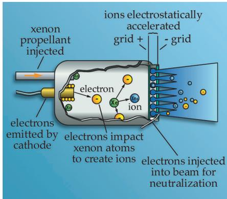
**Figure 4.2.1-37. Simple Ion Thruster.** An ion thruster is the simplest example of an electrodynamic rocket. A strong electric field accelerates an ionized propellant to high velocity (>30 km/s). To prevent charging of the spacecraft, negative ions are injected into the exhaust, neutralizing it.
