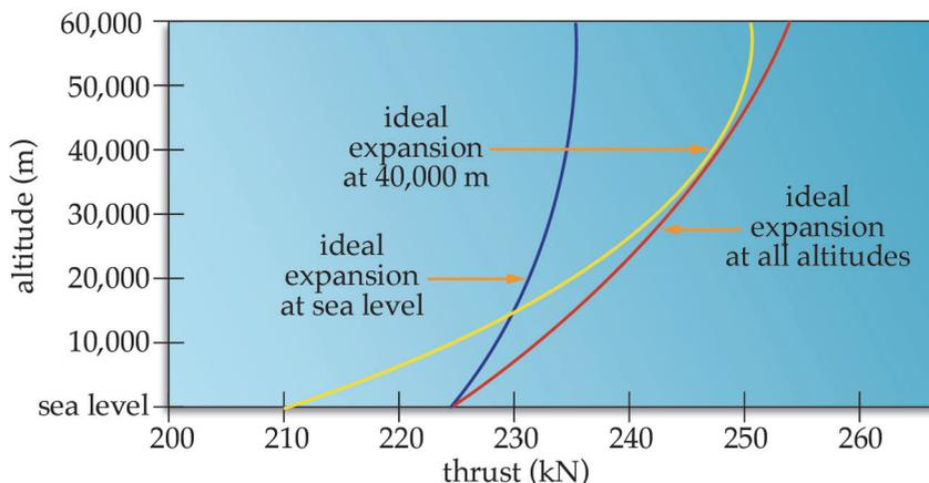
**Figure 4.2.1-52. Thrust Versus Altitude for Different Nozzle Designs.** Because we can't build an ideally expanded nozzle for all altitudes, we typically design them for ideal expansion 2/3 of the way up. In this example, we design a nozzle that must work from sea level to 60,000 m altitude for ideal expansion at 40,000 m. This design offers better overall performance than a nozzle designed for ideal expansion at either sea level or 60,000 m.
