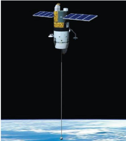
**Figure 4.2.1-47. Tether Experiment.** This artist's concept shows a small mass deployed downward on a long tether. (Courtesy of NASA/Marshall Space Flight Center)
