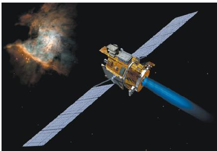
**Figure 4.2.1-38. Ion Engines in Space.** NASA's Deep Space 1 mission used an ion thruster for its primary propulsion. The engine operated at 2.3-kw, producing a thrust of 0.09 N with a specific impulse of 3100 s. (Courtesy of NASA/Jet Propulsion Laboratory)
