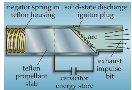
**Figure 4.2.1-41. Pulsed-plasma Thruster (PPT).** PPTs create a plasma by pulsing an electric arc over the surface of a solid propellant, such as Teflon (PTFE). The induced magnetic field accelerates the plasma. As the teflon slab shrinks, the negator spring gradually feeds it into the arc.
