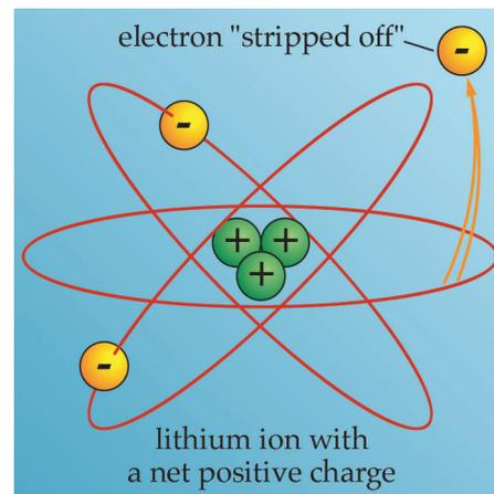
**Figure 4.2.1-7. An Ion.** We create an ion when we “strip off” outer-shell electrons from a neutral atom or molecule, leaving a net positive charge. Electric or magnetic fields can then accelerate this ion.
