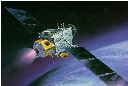
**Figure 4.2.1-34. Arcjets at Work.** The Argos spacecraft, shown here, tested a powerful 26-kW ammonia ( $\text{NH}_3$ ) arcjet, setting a record for the most powerful electric-propulsion system ever tested in orbit. Its  $I_{sp}$  was 800 s, and its thrust was 2 N. (Courtesy of the U.S. Air Force)
