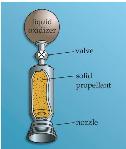
**Figure 4.2.1-28. Hybrid Rocket Motor.** A hybrid rocket uses a solid fuel with a liquid oxidizer. This offers the flexibility of a liquid system with the simplicity and density of a solid motor. Falling in between liquids and solids in performance, hybrids have yet to see applications on launch vehicles or spacecraft.
