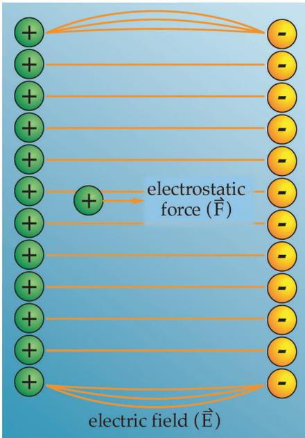
**Figure 4.2.1-14. Electrostatic Force.** An electric field exists when there is an imbalance between positive and negative charges in a confined region. This field will place an electrostatic force on a charged particle within the field, accelerating it.
