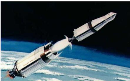
**Figure 4.2.1-56. Saturn I during Staging.** When a launch vehicle, such as the Saturn I shown here in an artist's concept, stages, it shuts off the lower-stage rocket, separates it, and ignites the rocket on the next stage to continue into orbit. (Courtesy of NASA/Kennedy Space Center)
