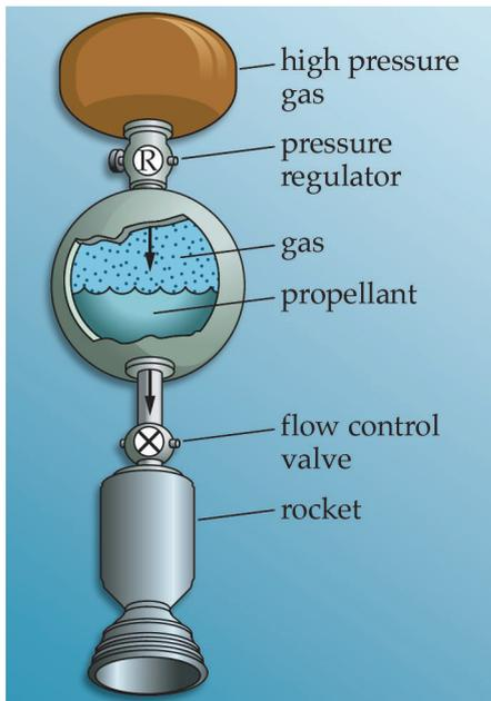
**Figure 4.2.1-16. Pressure-fed Propellant System.** In a pressure-fed propulsion subsystem, high pressure gas forces the liquid propellant into the combustion chamber under pressure, much like blowing liquid through a
