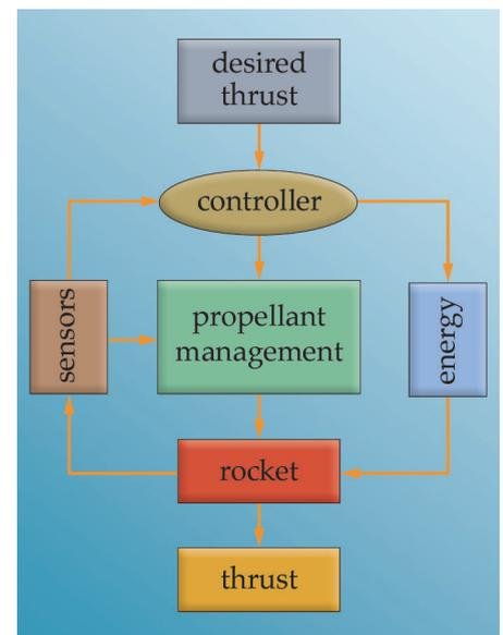
**Figure 4.2.1-15. Block Diagram of a Complete Propulsion Subsystem.** A propulsion subsystem uses the desired end state (specific thrust at a specific time), plus inputs from sensors, to determine commands for propellant management and energy control that produce the system output—thrust.
