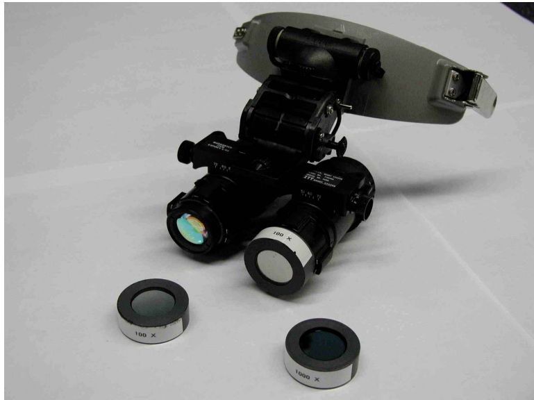
Fig. 9 F4949 night vision goggles with 2ND filters. In combination with the gelatinous filter in front of the collimated display, the NVGs can be used for training in the DISO.
