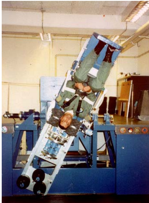
Fig. 4 The 3-D chair in roll mode. Demonstration of leans and ferriswheel illusion.
