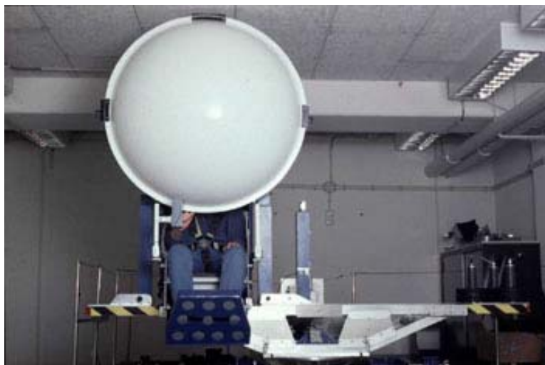
Fig. 3 Excentric mode of 3-D rotating chair. Demonstration of somatogravic effect and interaction with visual stimuli.
