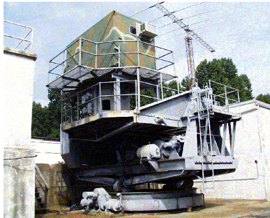
Figure 3: Naval Research Laboratory's Ship Motion Simulator (SMS). Capable of +/- 14 degrees pitch; +/-5 degrees roll, 8 s period.
