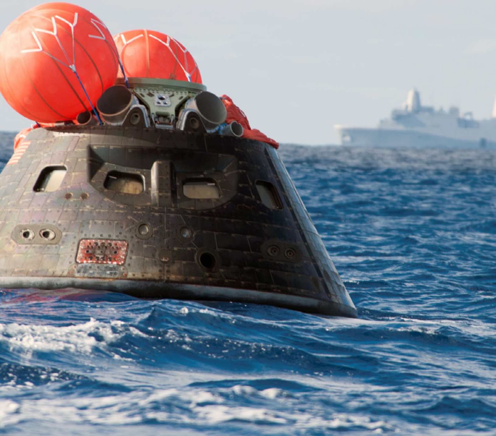
NASA's Orion spacecraft floats in the Pacific Ocean after splashdown from its first flight test in Earth orbit, to test systems critical to crew safety, including the launch abort system, the heat shield and the parachute system. December 5, 2014, San Diego, California. Photo credit: NASA/Tony Gray
