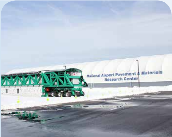
A heavy vehicle simulator used for runway pavement research at the FAA’s National Airport Pavement & Materials Research Center at the William J. Hughes Technical Center in New Jersey.
