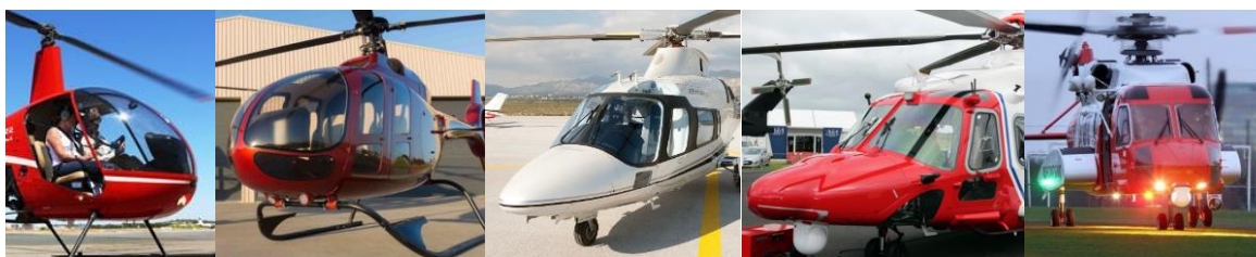
Figure 22. Comparison of windshields on R22 (Part 27 Tier I), EC120 (Part 27 Tier II), A109 (Part 27 Tier III), AW-189 (29.631), and S-92A (29.631).
