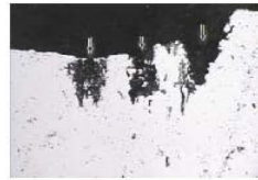
Photo of pitting in taper bore surface
