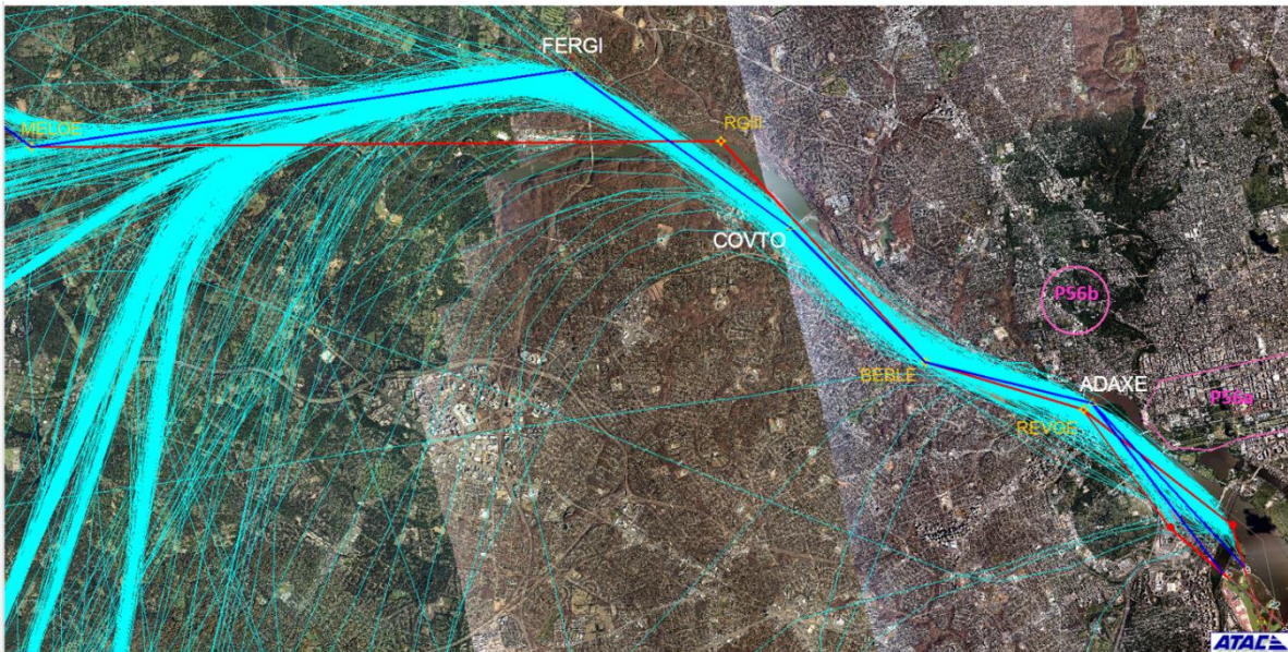
Figure 1: The blue line represents the current air traffic route and the red line represents the proposed amended route, removing waypoint FERGI and adding the new waypoint RGIII.
