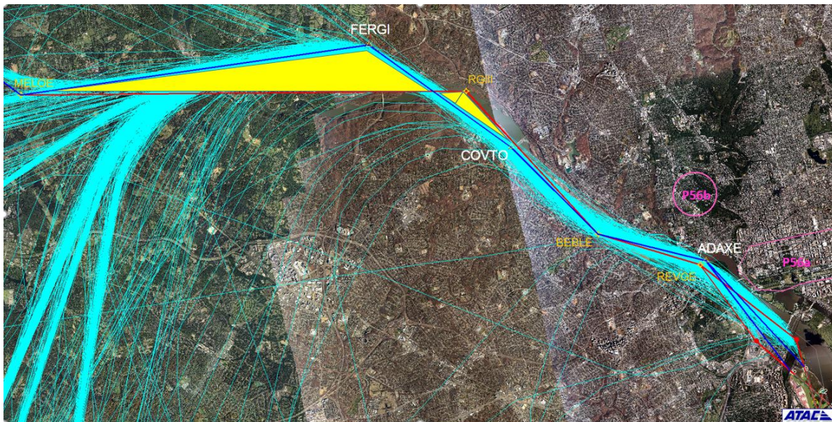
Figure 3. The APE is depicted by the yellow highlighted areas. The blue line is the current route and the red line is the proposed route. Light blue lines are radar tracks for aircraft using the current route.
