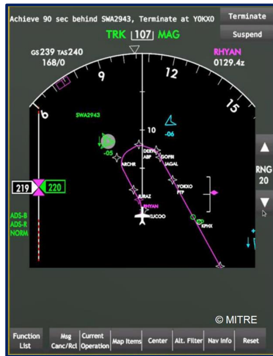
Figure 5. CDTI for IM application (prototype used in MITRE HITL experiments).
