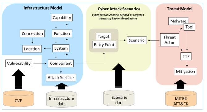
The CICAT data model includes data imported as XML files (CVE and ATT&CK for Industrial Control Systems (ICS)), as JSON files (Enterprise ATT&CK), and as Excel spreadsheets (Infrastructure and scenario data).
