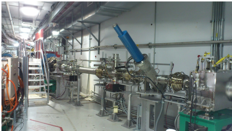
Figure 9. Beam transport to the RID, which is off to the right. (the stripping foil equipment is behind the stairs; this is the highest dose rate region of the accelerator)
