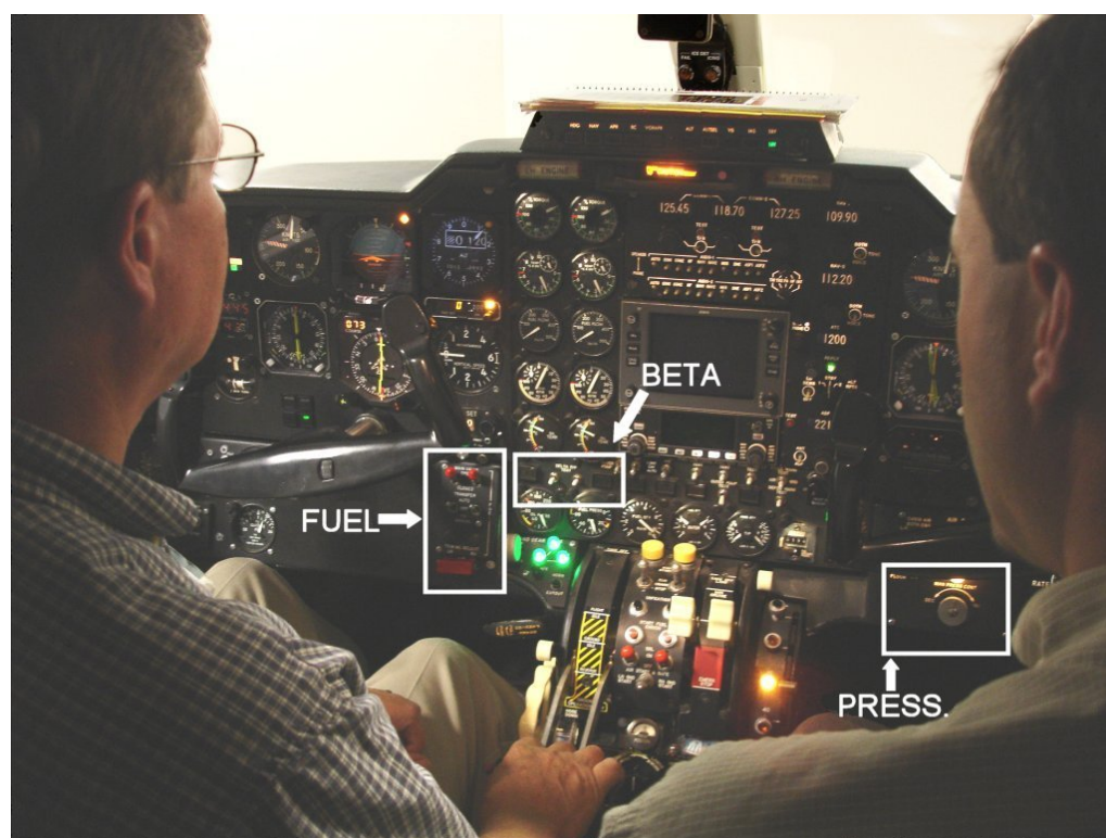
Figure 1. Overview of instrument panel showing location of fuel switches, beta lights and pressurization control.
