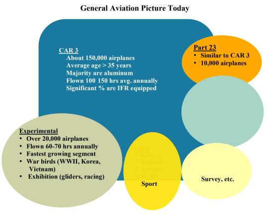
The FAA is responsible for overseeing the continued airworthiness of more than 150,000 type-certificated GA airplanes over 30 years old. Most of these airplanes were designed to Civil Air Regulations (CAR) 3 standards established in the 1950s or earlier and were produced before the 1980s. A small portion of the fleet is designed to early design standards – Aero Bulletin 7a, CAR 4, and CAR 4a. Many are vintage airplanes designed or produced before World War II.
