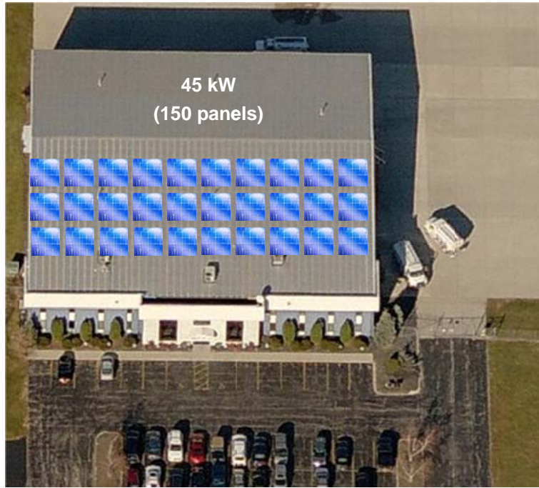
Illustration of approximately 45 kW of PV panels on the FBO building roof. Each square represents 6 panels.
