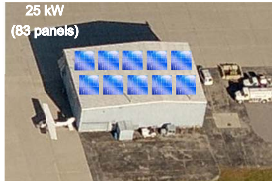
Illustration of approximately 25-kW of PV panels on the FBO Hangar roof (near the ARFF building). Each square represents 6 panels.
