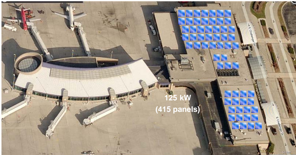
Illustration showing approximately 125 kW of PV panels installed on the Passenger Terminal roof. Each square represents 6 panels.
