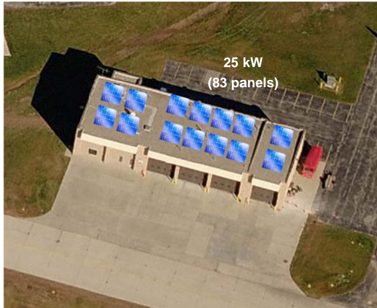
Illustration of approximately 25-kW of PV panels on the ARFF building roof. Each square represents 6 panels.
