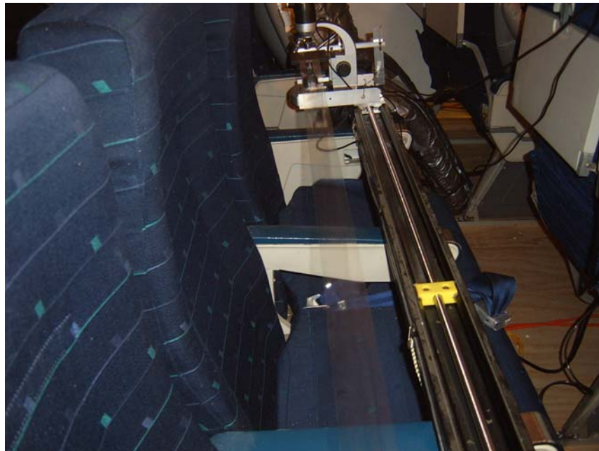
Figure 12.3 Microscope traversing system.
