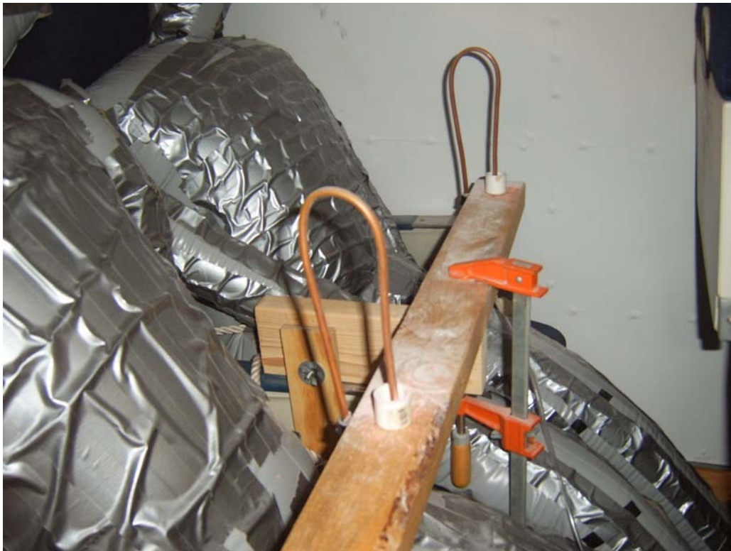
Figure 12.1 Dust injection apparatus
