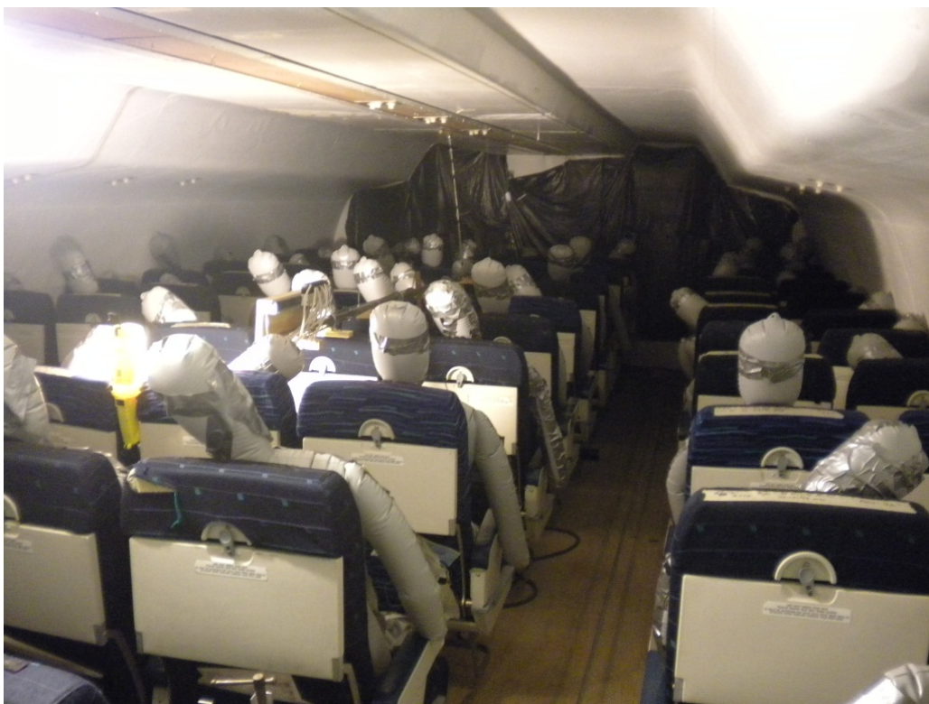
Figure 11.1 Eleven-row mockup of the interior of a Boeing 767 cabin.
