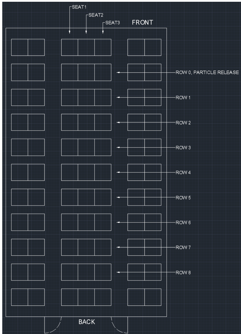
Figure 12.6 Cabin layout and nomenclature for experiments.
