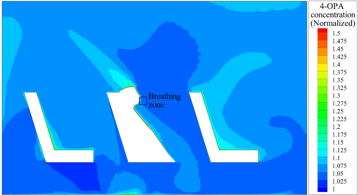
Figure 6.6. The 4-OPA distribution in the longitudinal section through center of the occupied cabin mockup with an outdoor air change rate of 4.4 \text{ h}^{-1} for Case 3.
