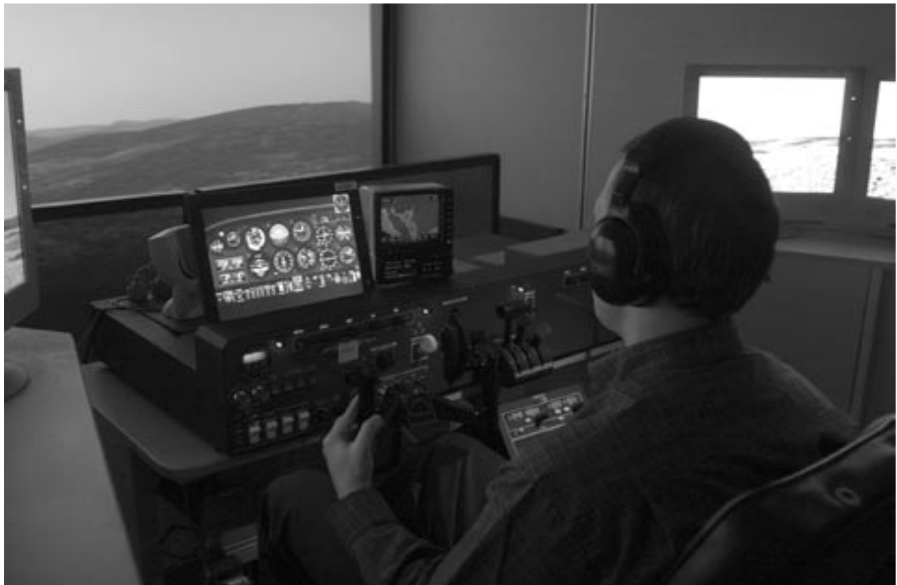
Figure 2: Basic General Aviation Research Simulator (BGARS).
