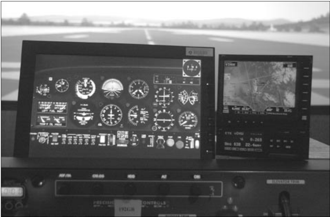
Figure 3. Close-up view of the BGARS aircraft instruments and GPS/MFD displays (to the right).
