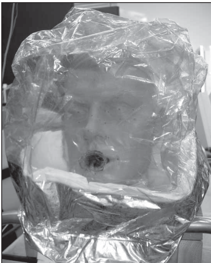
Figure 1. The Emergency Passenger Oxygen System evaluated in this study. The unit contains a single oxygen cylinder (not visible) that is normally opened to the interior of the unit when taken from the packaging for donning.
