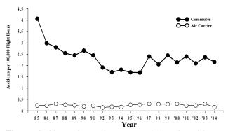
**Figure 1.** Air carrier and commuter/air taxi accident rates since 1985 (Source: NTSB).
