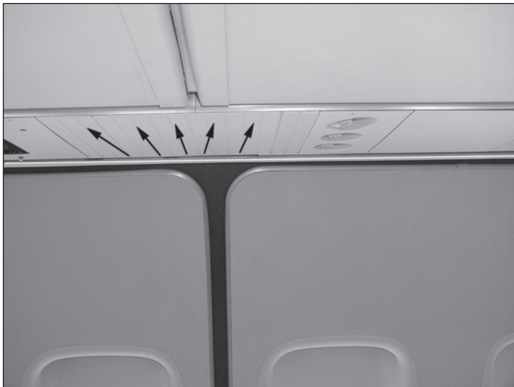
Figure 3. Graphic illustrating Boeing 747 ECS cabin ventilation supply plenum air introduction into passenger cabin. View facing cabin sidewall intersection with overhead luggage carrier.
