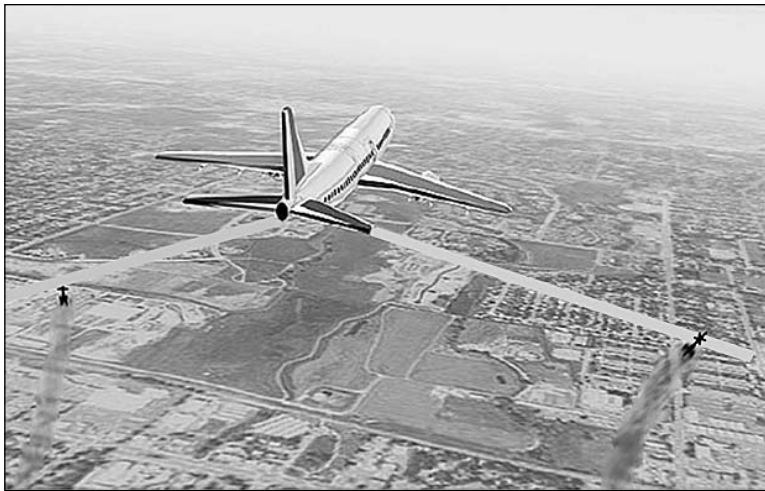
Figure 7. Conceptual illustration of a civilian Counter-MAN-PADS deploying (invisible) IRCM to disrupt the guidance systems of surface-to-air missiles.
