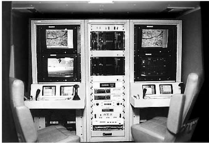
Figure 4. Predator control station.
