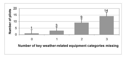
**Figure 7.** Numbers of non-IR pilots (vertical axis) lacking one or more categories (horizontal axis) of either weather-avoidance electronics, de-icing capability, and/or autopilot/winglever.
