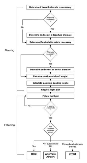
Figure 2. A Generalized View of the Dispatch Process
