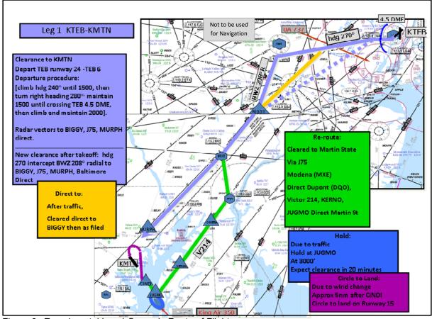
Figure 2. Experimental Leg 1 Scenario Route of Flight.
