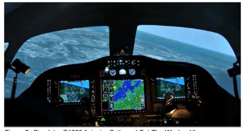
Figure 6. Simulator G1000 Avionics Suite and Out-The-Window View.
