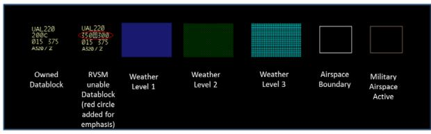
Figure 2. ERAM. Example of Color Coding for ATCOV 6.1, Including RVSM, Weather, and Military Space
