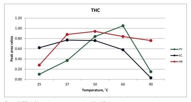
**Figure 7.** Effect of incubation temperature on the ability of  $\beta$ -glucuronidase enzymes to hydrolyze THC-glucuronide.
