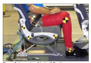
Figure 8. Lower Leg "Vertical" Position
