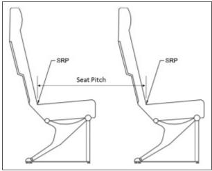
Figure 12. Seat to Seat Configuration
