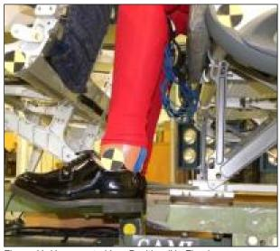
Figure 11. Unsupported Leg Position (No Floor)
