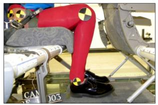
Figure 10. Lower Leg "Aft" Position
