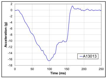
Figure 3 – Typical Sled Deceleration Pulse
