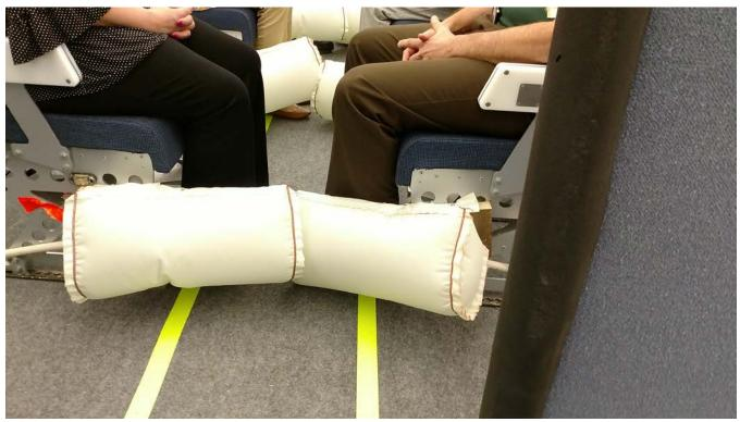
Figure 2: Airbags fully deployed with participants; the picture was taken from just outside forward opening of mock-up.
