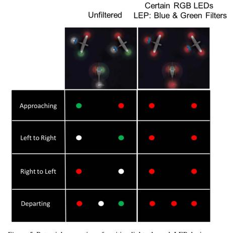
Figure 5. Potential perception of position lights through LEP devices
