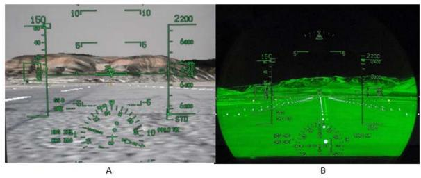
Figure 2. The head-down primary flight display (HDPFD) (A) and the head-up display (HUD) (B).
