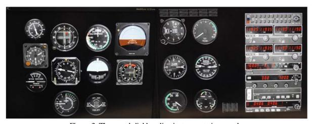
Figure 3. The round-dial baseline instrumentation panels.
