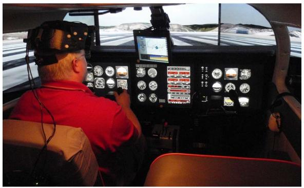
Figure 8. The Advanced General Aviation Research Simulator (AGARS) configured as a Piper Malibu/Meridian with the HUD stowed and pilot using the HMD.
