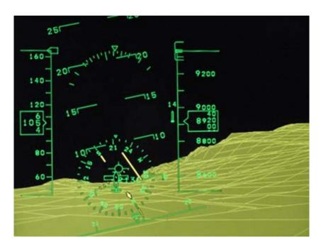
Figure 11. HMD wire-frame version of terrain image.
