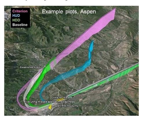
Figure 6. One set of tracks, one individual, for approaches to Aspen/Pitkin County showing the criterion track (magenta) and the three experimental trials.
