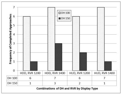
Figure 4. Frequency of completed approaches/landings by DH, RVR, and display type.
