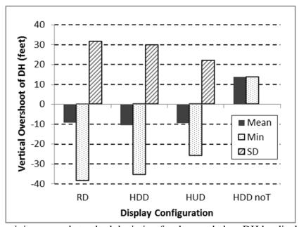
Figure 5. Mean, minimum, and standard deviation for descent below DH by display type where RD = round dial, HDD = head-down display, HUD = head-up display, and HDD noT = head-down display without terrain. Task 2, Full-mission simulation from KEGE to KASE
