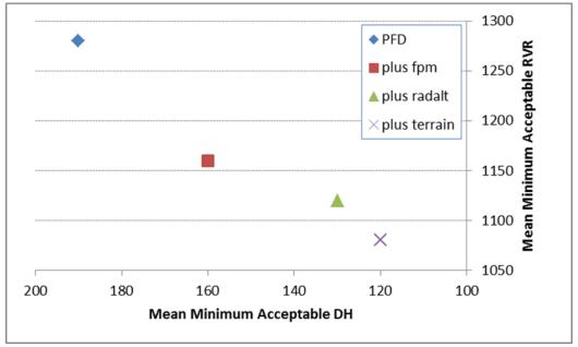
Figure 7. Means of responses to the question regarding what minima pilots would accept for each addition to the basic HMD with PFD equipment configuration.
