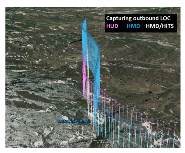
Figure 16. Example effect of HITS guidance in HMD on acquiring outbound course.
