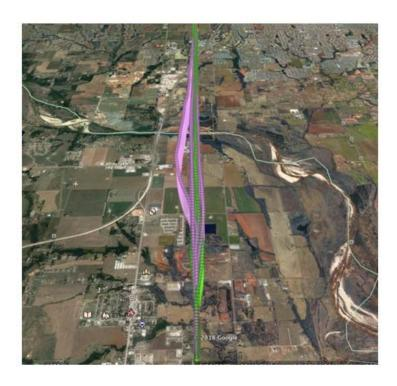
Figure 13. Track dispersion on approach with SV present on the displays.
