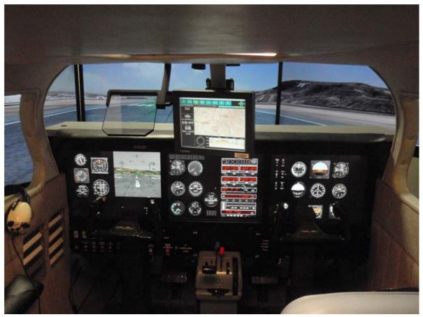
Figure 1. The Advanced General Aviation Research Simulator (AGARS) with HD, EPFD, HUD, and electronic map
