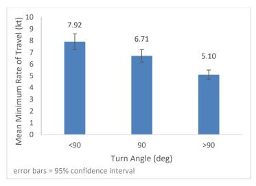
Figure 12. Mean minimum rate of travel during turns by turn angle (Study 1).
