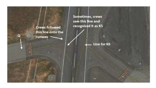
Figure 4. Layout of intersection 2 and lead-on/lead-off lines.
