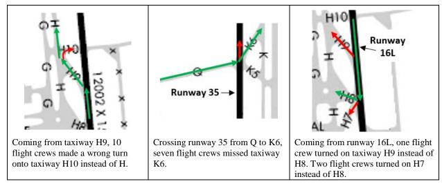
Figure 2. Intersections with common route deviations (Study 1). Note: Routes in green, deviations in red.
