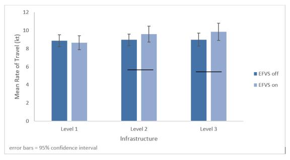
**Figure 10. Mean rate of travel by EFVS and infrastructure (Study 1).** Note: Statistically significant post-hoc comparisons (LSD, p < .05) are represented by a line connecting the bars.
