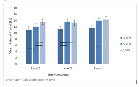
Figure 26. Mean rate of travel by RVR and infrastructure (Study 2). Note: Statistically significant post-hoc comparisons (LSD, p < .05) are represented by a solid line connecting the bars. The dashed line
