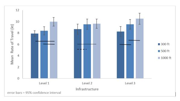
**Figure 11. Mean rate of travel by RVR and infrastructure (Study 1).** Note: Statistically significant post-hoc comparisons (LSD, p < .05) are represented by a solid line connecting the bars. The dashed line represents a moderately significant difference (p < .10).
