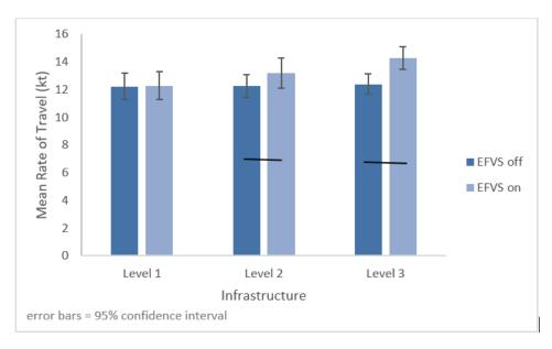
**Figure 25. Mean rate of travel by EFVS and infrastructure (Study 2).** Note: Statistically significant post-hoc comparisons (LSD, p < .05) at each level of infrastructure are represented by a line connecting the bars.
