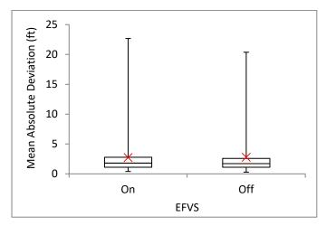
Figure 6. Centerline deviations by EFVS condition (Study 1) showing mean (red X), 25<sup>th</sup>, 50<sup>th</sup>, 75<sup>th</sup> percentiles (box limits), and range (vertical line extent).
