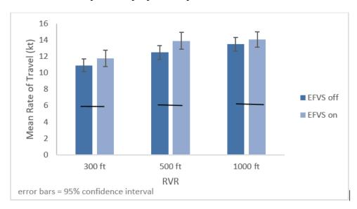
Figure 24. Mean rate of travel by EFVS and RVR (Study 2). Note: Statistically significant post-hoc comparisons (LSD, p < .05) at each level of RVR are represented by a line connecting the bars.
