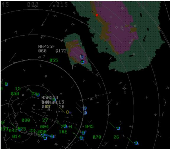
*Figure 5.* HF-STD-010-compliant rendition of STARS with all 3 standard weather colors plus black stippling used to show severities 1 through 6.
