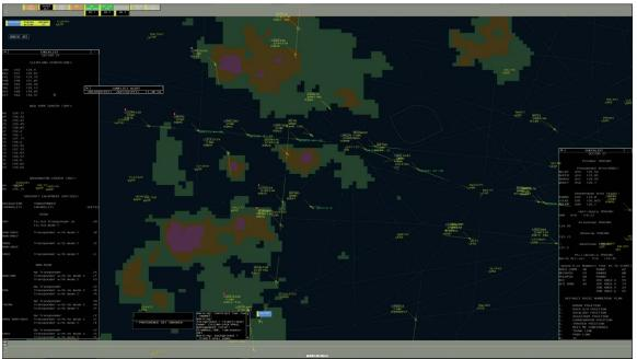
*Figure 4.* HF-STD-010-compliant rendition of ERAM with all 3 standard weather colors used to show severities 1 & 2, 3 & 4, and 5 & 6.
