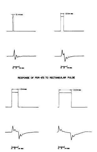
Figure 1. Response of PDR-8 earphone to 0.1-, 0.5-, 1.0-, and 2.0-ms rectangular current pulses.
