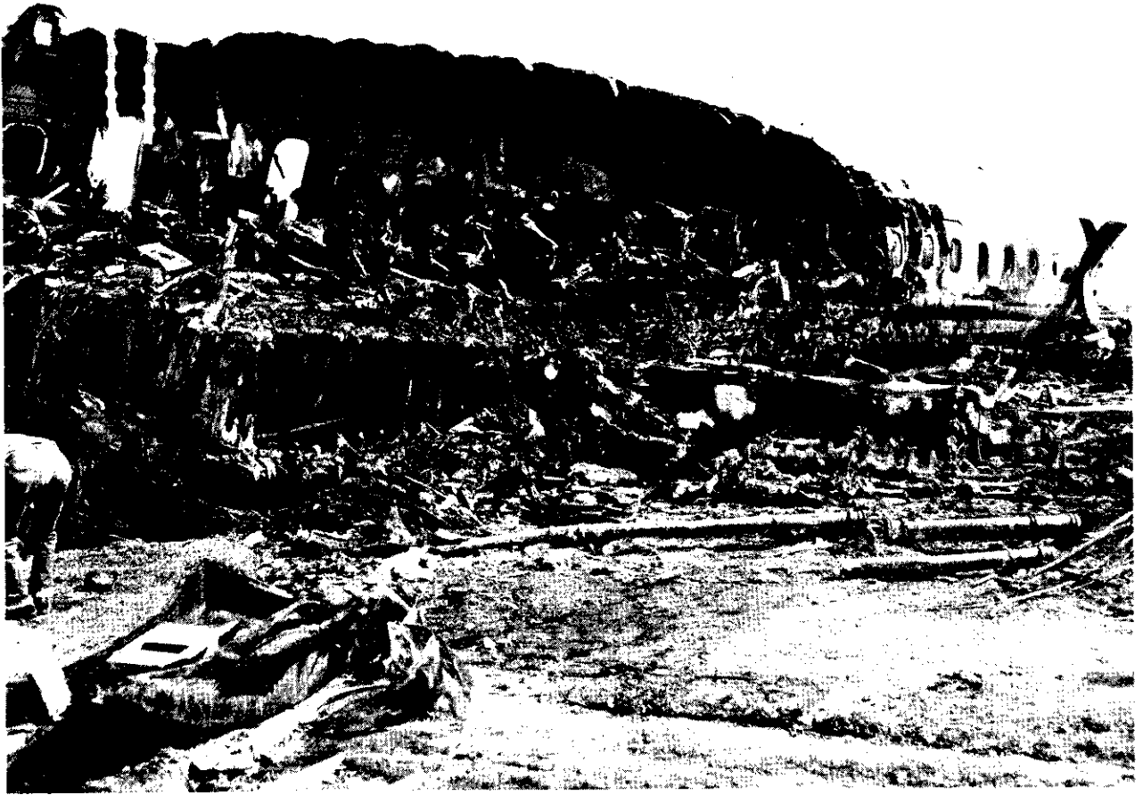
FIGURE 7. Post-fire view of Denver DC-8 from left front. The #1 (left outboard) engine was detached and impacted beneath the left wing root. The resulting fire was initially limited and did not penetrate the cabin until evacuation was complete. It later flared out of control and extensively damaged the aircraft interior.
