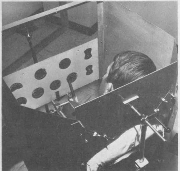
FIGURE 1. Modifications of a rotating device to control head movements and to introduce an aviation-related visual environment. The rod extending upward from the foot rest terminates in a plastic panel which contains three tiny lights (a red and a green "wing-tip" light and a flashing red "beacon") simulating an approaching aircraft. Upper left: rotation device without the "cabin" attachment (the chin rest depicted here is used for research rather than demonstration purposes). Upper right: the major section of the "cabin" has been bolted to the back of the head rest; its base is further supported by small metal extensions projecting outward from the arms of the chair. Lower left: the instrument panel is added to the "cabin" by means of four wing-nuts. Lower right: interior view of the "cabin" with a subject's head tilted to the right; the lights of the approaching aircraft were viewed through the "window" of the "cabin." The interior of the "cabin" was coated with luminous paint.
