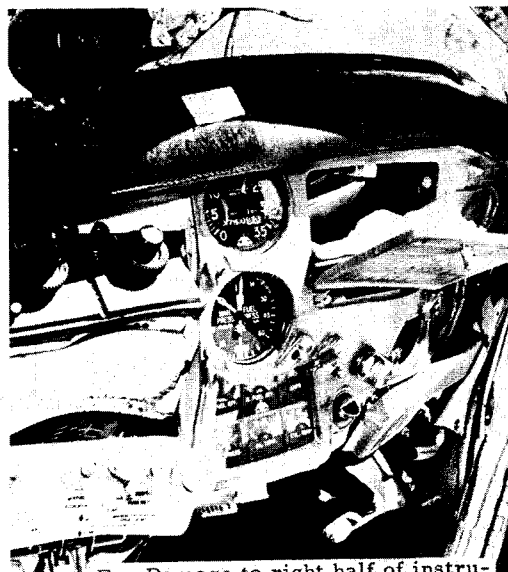
F. Damage to right half of instrument panel from unrestrained stretcher.
