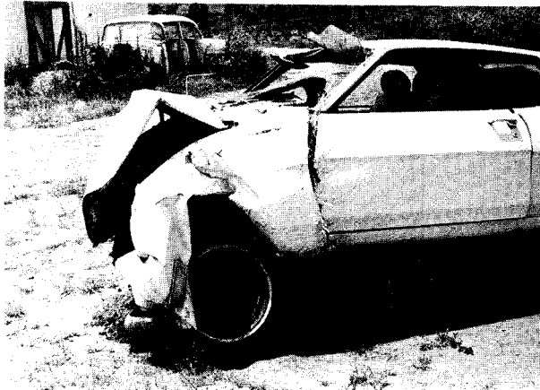
FIGURE 30. Side view of vehicle showing crushing of front end during deceleration.
