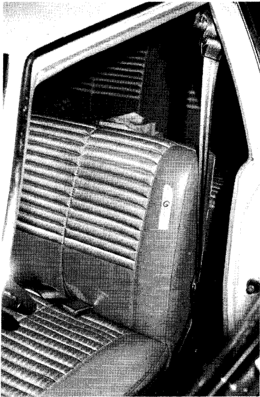
A Shoulder strap and half of lap belt held neatly vertical along B post by two retractors. Only one buckle in seat.
