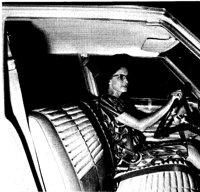
C Subject wearing three-point belt restraint system.
