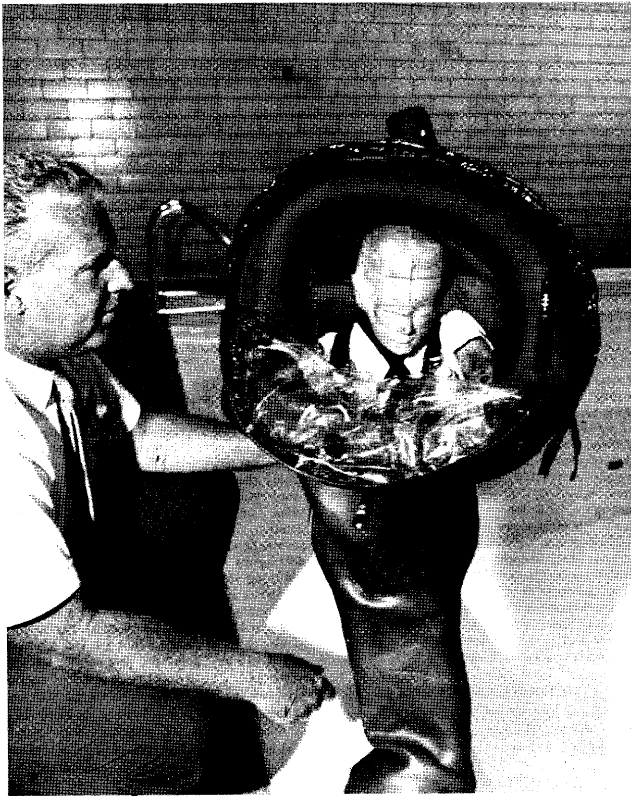
FIGURE 1. Initial prototype of the infant flotation device occupied by a child anthropomorphic dummy.
