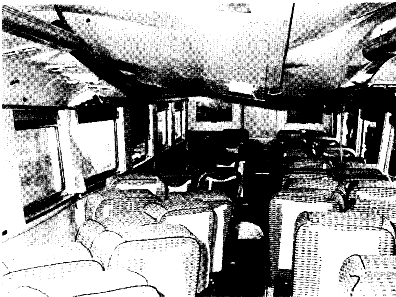
b. All seats on the left side of the car are unhooked and rotated aisle side forward approximately 45^{\circ} . This rotation may have protected some passengers to a degree as some were trapped in their seats and not thrown to the opposite side of the car.
