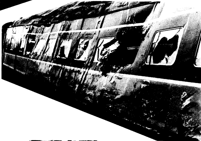
b. One passenger was killed when a cross-tie came into the car through the hole near the center of the picture.
