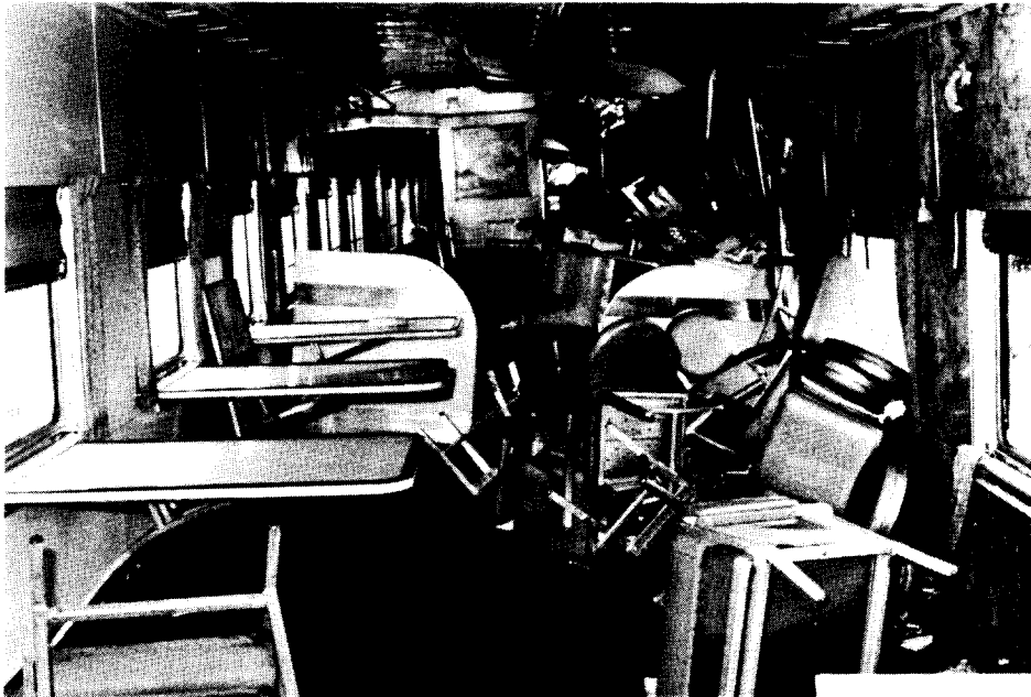
b. Same view as a above except that the car has been righted. At least two passengers were ejected through one of the windows in the right of the picture.
