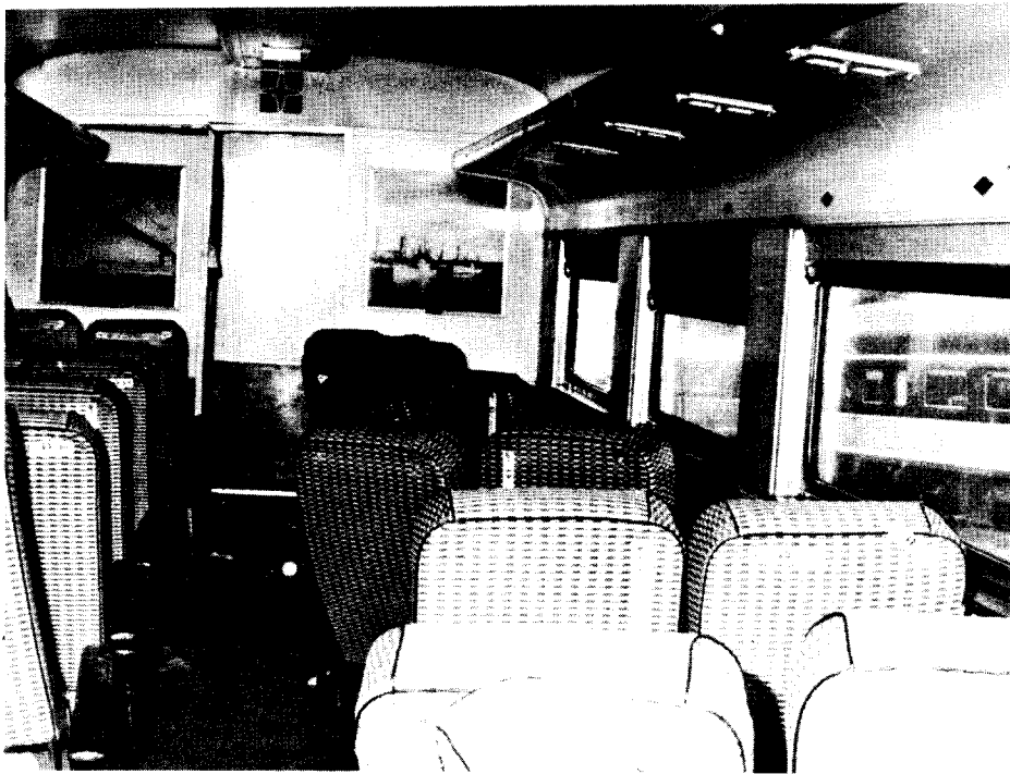
a. Right forward section--very minor damage--seats rotated.
