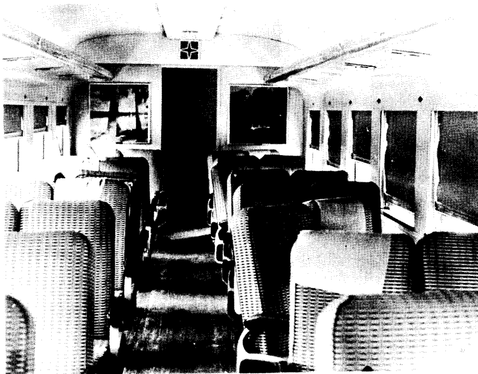
b. Even though the car remained upright, some seats became unhooked and rotated. The passengers in these cars stated they were able to remain in their seats by holding on.
