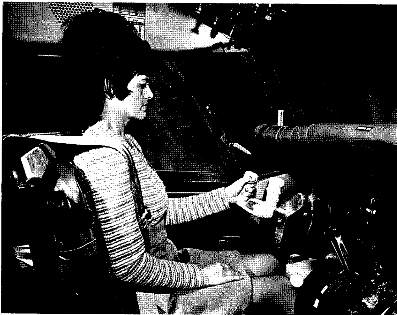
FIGURE 3. Modified seat and wheel; note permanent seat cushion, shoulder harness and subject's grip on Bonanza wheel.
