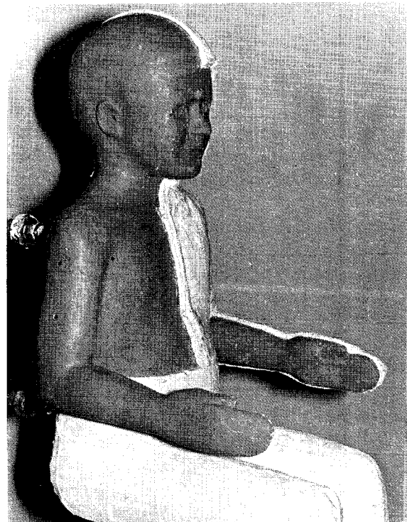
FIGURE 3.—Six-year-old-child masterbody form in the process of mold casting.
