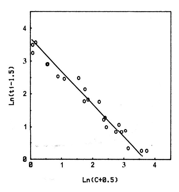
Figure 5. Loq-log plot of  $(t_1-1.5)$  versus (C+0.5), a linearized transformation of Fig. 3. Fitted regression equation: ln(t-1.5) = ln(40) - ln(C+0.5).
