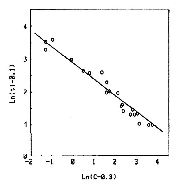
Figure 9. Log-log plot of (t<sub>1</sub>-0.1) versus J(C-0.3), a linearized transformation of Fig. 7. Fitted regression equation:  $ln(t_1-0.1) = ln(18) - \frac{1}{2}ln(C-0.3)$ .
