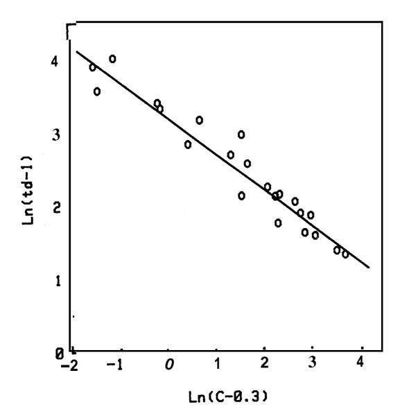
Figure 10. Log-log plot of (t<sub>d</sub>-1.0) versus J(C-0.3), a linearized transformation of Fig. 8. Fitted regression equation:  $ln(t_d-1.0) = ln(25) - 4ln(C-0.3)$ .
