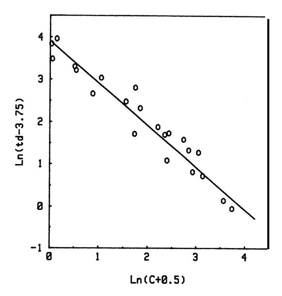
Figure 6. Log-log plot of (t<sub>e</sub>-3.75) versus (C+0.5), a linearized transformation of Fig. 4. Fitted regression equation:  $ln(t_e-3.75) = ln(50) - ln(C+0.5)$ .
