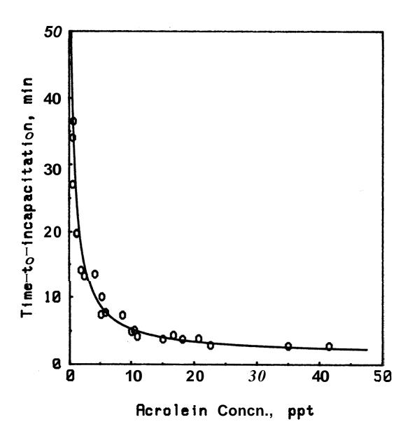
Figure 3. Time-to-incapacitation as a function of the average chamber concentration of acrolein. Fitted regression equation:  $t_1 = 1.5 + 40/(C+0.5)$ , RSSQ = 238.
