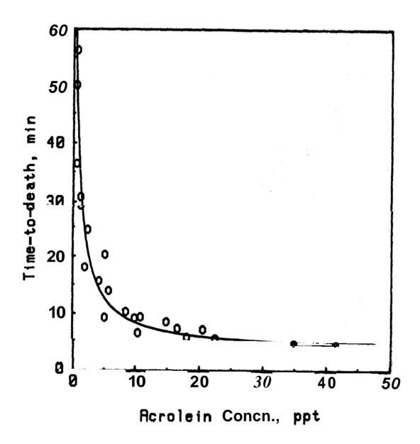
Figure 4. Time-to-death as a function of the average chamber concentration of acrolein. Fitted regression equation:  $t_d = 3.75 + 50/(C+0.5)$ , RSSQ = 473.
