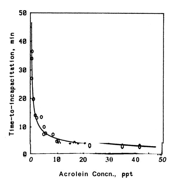
Figure 7. Time-to-incapacitation as a function of the square root of the effective acrolein concentration. Fitted regression equation:  $t_1 = 0.1 + 18/J(C-0.3)$ , RSSQ = 141.
