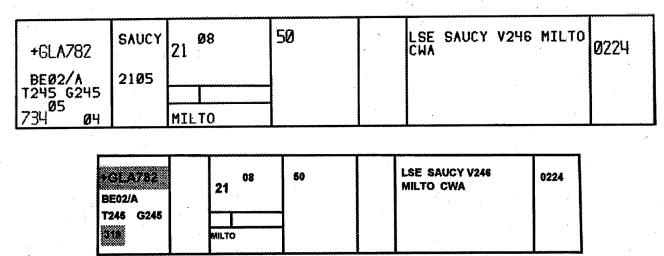
**Figure 1**. Examples of flight progress strips used in this study. On top is the flight progress strip (FPS) used today. On the bottom, is the 1" x 5" reduced flight progress strip (RFPS), which has the call sign and computer ID in bold.
