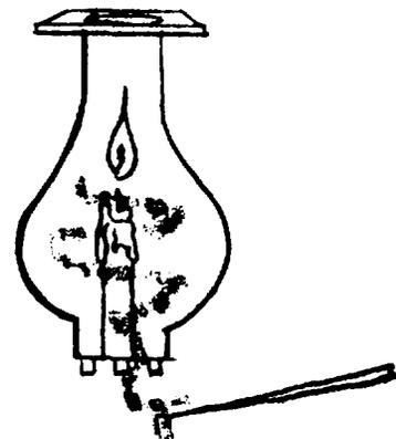
Light the candle and place the chimney over it, resting the chimney on sticks so that air can circulate under the edge. Put the cover glass over the top of the chimney. Light the splinter and hold it near the base of the candle so that smoke will circulate inside the chimney.
