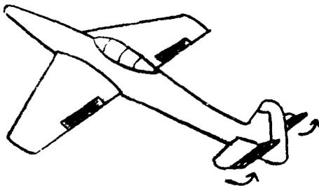
When the pilot wants his plane to climb, he moves his controls so that the elevators tilt up in the same way that you folded the back edges of the glider. The air hitting the elevators pushes the tail of the plane down, tilting the nose upward, so that the plane can climb.
