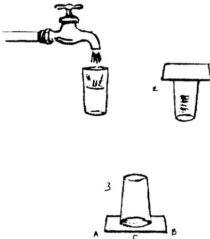
At A and B the upward and downward pressures balance, but at C the upward pressure of air is greater than the downward pressure of water and holds the cardboard in place.
