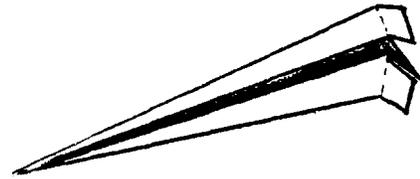
b. *Right and left.* Turn the vertical fin on the glider a little to the right; the glider will fly toward the right. The pilot moves his rudder to the right for a right turn, but he must also bank his plane for the turn, the same as you would do if you were turning on a bicycle. (You would lean to the right for a right turn.) The pilot tilts his plane to one side by using the ailerons. When one tilts up the other tilts down.
