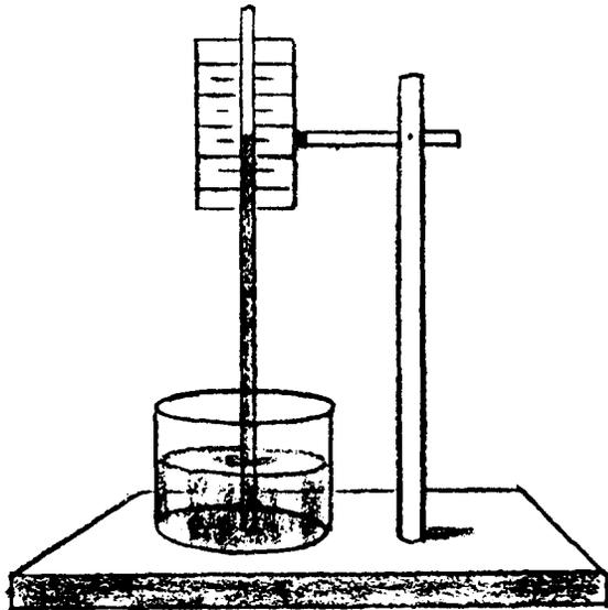
Mark a scale of inches and half inches on the cardboard, and label it from 24 to 36 inches. With the yardstick, measure the actual height of the mercury column and attach the scale to the proper spot on the tube.
