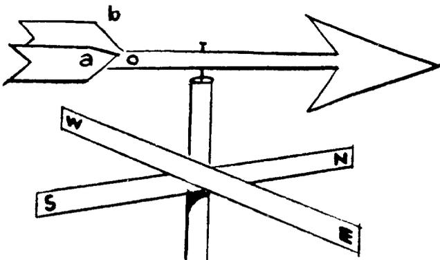
Cut arrow and shaft from 20" strip. Cut tailpieces from 8" strips. Nail them to shaft of arrow on each side; spread them apart to form an angle of 200 in order to catch the wind easily, using a protractor to measure the angle  $AOB$  (see illustration). Find the balance point by resting shaft on extended finger until arrowhead and tailpieces balance level; drill hole at this point. Insert long nail in hole. Place bead on nail to act as bearing. Mount on post, preferably away from buildings.
