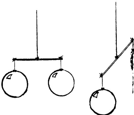
Blow up the balloons to the same size, and tie them at their necks with a piece of string. Tie one balloon to each end of the dowel stock. Attach another piece of string to the center of the dowel stock and suspend it from some convenient place. Balance the dowel stock. Prick one balloon with a pin. As the air rushes out, the pricked balloon shoots up and the heavier, air-filled one drops down.
