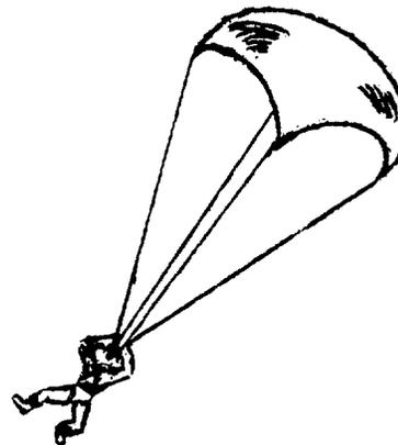
A parachute floats' downward toward the earth through the air. When an object falls from a great height it picks up speed, but the resistance of air finally causes it to fall at a steady speed called *terminal velocity*. The large surface of a parachute acts as an air brake, checking the velocity of the person or object attached and making possible a safe landing.
