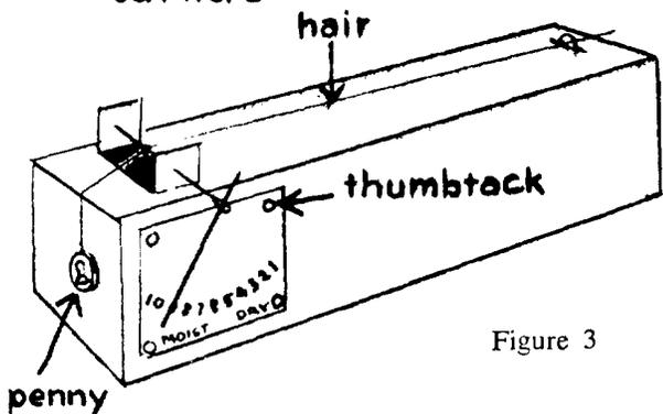
Tie the hair to the paper clip, wind it around the needle, tape the penny to the other end of the hair, and let the penny hang over the end of the box, which should be lying on its side.
