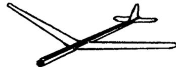
The glider does not have a propeller or a motor. When you toss the glider into the air, the air pushes up on the wings. This pressure keeps the glider from coming straight down.
