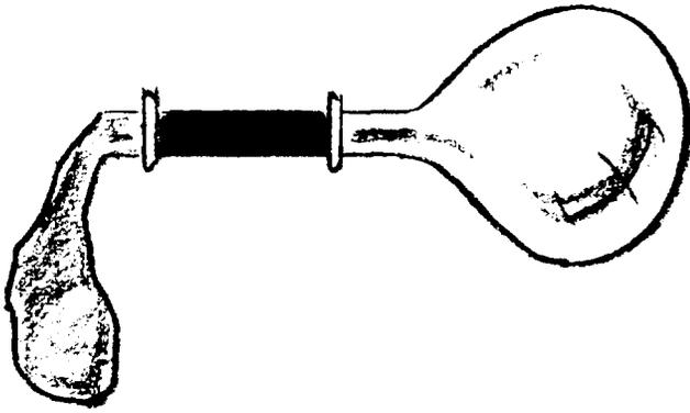
Air rushes from the inflated balloon to the empty balloon. When the air pressures inside the two balloons become equal, the air stops moving from one to the other. Are they now the same size?
