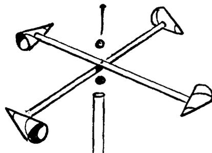
The anemometer may be calibrated with a fair degree of accuracy as follows: Hold it out the window of an automobile moving at a constant rate of speed. Note the speedometer reading and the distance traveled and the revolutions per minute (rpm) of the anemometer. Drive the car back along the same road and note the same readings, being sure the speed of the car and the distance traveled are the same as before. Average the 2 rpm counts to allow for the effect of any wind.
