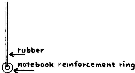
Fasten this end to the glider as shown in the diagram below; then anchor with a pin. Even kindergarten children can use this method of suspending a glider in a wind tunnel. (See No. 55.)
