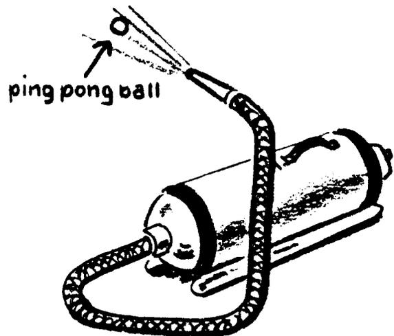
up. Release the ping-pong ball into the stream of air about a foot from the nozzle. Slowly tip the nose so that the air shoots at an angle. The ball will stay suspended in the airstream. The force of gravity upon the ball tends to make it drop out of the airstream. However, the fast moving airstream lessens the air pressure on the portion of the ball remaining in the airstream, overcoming the force of gravity, with the result that the ball remains suspended.
