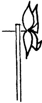
Experiment to see whether there is any angle toward the wind at which you might hold your pinwheel without it spinning. When does it slow down? Is it when the plane of the blades is parallel to the wind? Each blade is an airfoil. Can you explain why? (See No. 42.)
