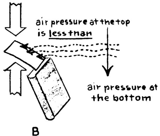
*Bernoulli's principle* states that an increase in the velocity of any fluid is always accompanied by a decrease in pressure. Air is a fluid. If you can cause the air to move rapidly on one side of a surface, the pressure on that side of the surface is less than that on its other side.
