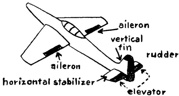
a. *Up and down.* Fold the back edges of the paper glider *up*, as in the diagram. When you throw the glider, the tail should go down and the nose should point up. It may take some practice to get the controls set so the glider does what you want it to do.
