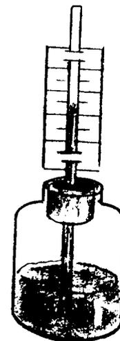
Note the temperature on an accurate thermometer. Record this temperature on the cardboard, which will act as a temperature scale. Place the thermometers in a different temperature situation and leave them for a few minutes to allow the thermometers to register the new temperature. Note the new reading and mark on the scale. Carefully measure the distance between the two readings on the scale, and mark other degrees of temperature on it, as all other changes will be in the same proportion.
