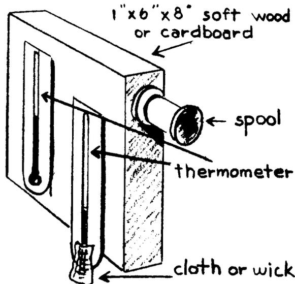
To make a sling psychrometer, remove the metal guard from one thermometer and cover its bulb tightly with the cloth or wick. Nail both the thermometers onto the board. Using the nut and bolt, attach the spool to the upper corner of the board, so that it will rotate freely.
