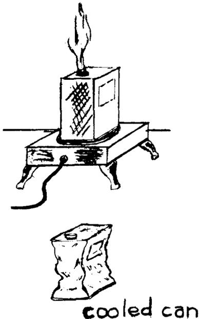
When it was heated water turned into steam, driving out most of the air. Now as the can cools, the steam turns back into water, leaving neither air nor steam inside the can. A partial vacuum has been created. Consequently, the pressure of air outside the can, being greater than that inside the can, crushes the can.
